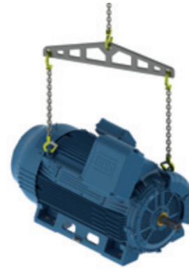
Figure 7 - Lifting with vertical chains.
